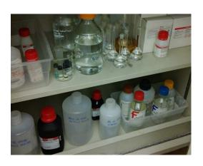
Sometimes we are limited on space, and it is hard not to store incompatibles next to one another. This photo demonstrates a good example of using spill trays to help consolidate chemicals that may be incompatible with others.
